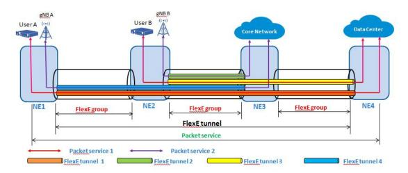
At Mobile World Congress Shanghai (MWCS) 2017, ZTE carried out an on-site test about the key technology FlexE Tunnel, including service isolation, ultra-low-latency forwarding, E2E OAM and fast protection switching. In this test, three 5G Flexhaul pre-commercial transport devices – ZXCTN 609 are used and connected with the tester (data tester IXIA XM2); the devices are networked by 100GE links.
