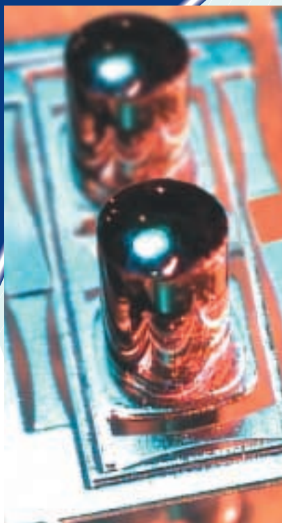
Detail showing collimators on MASS gimbal mounts in 64x64 switch core.
